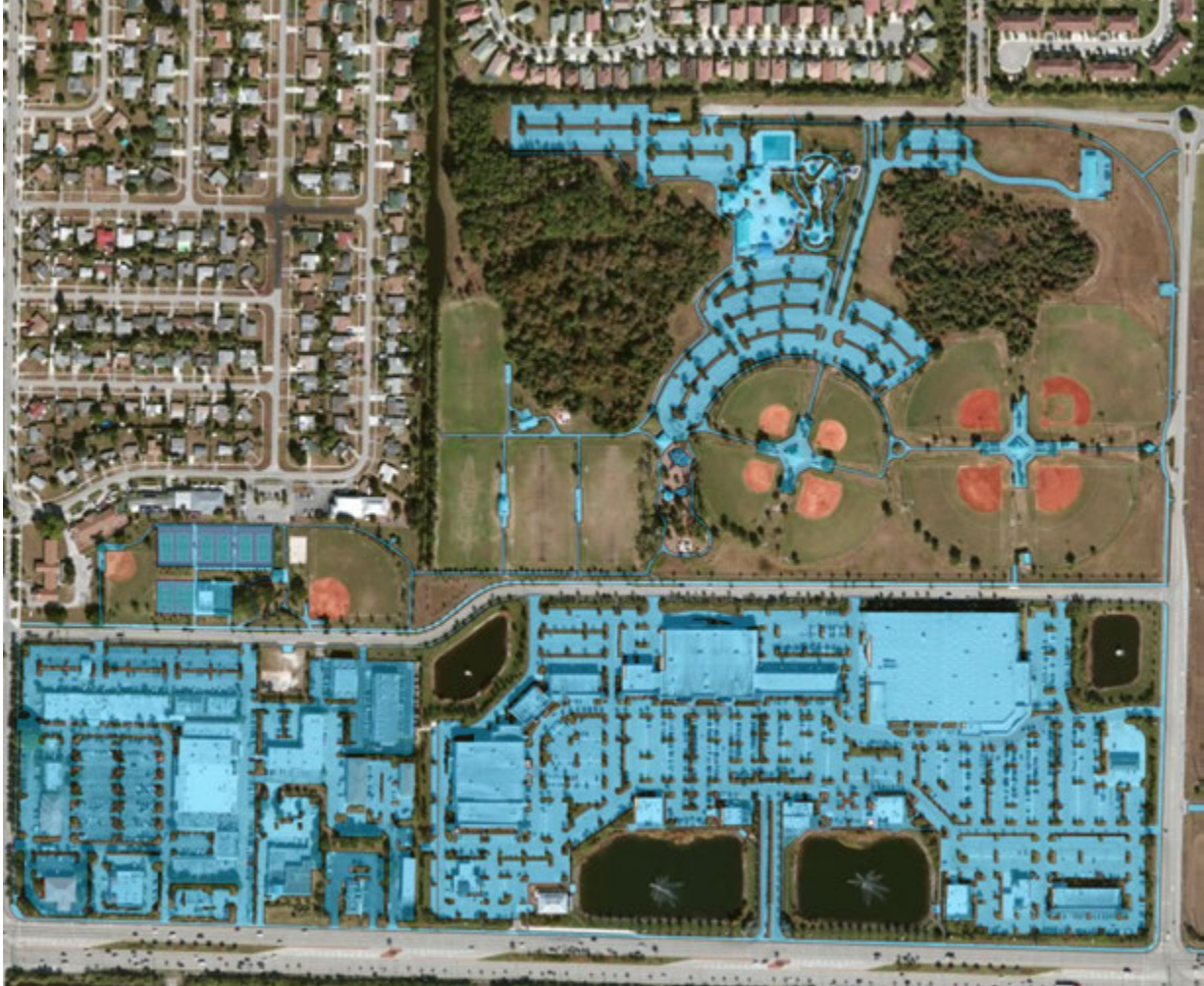
Figure 2-1 Nonresidential/Commercial Impervious Area Example
