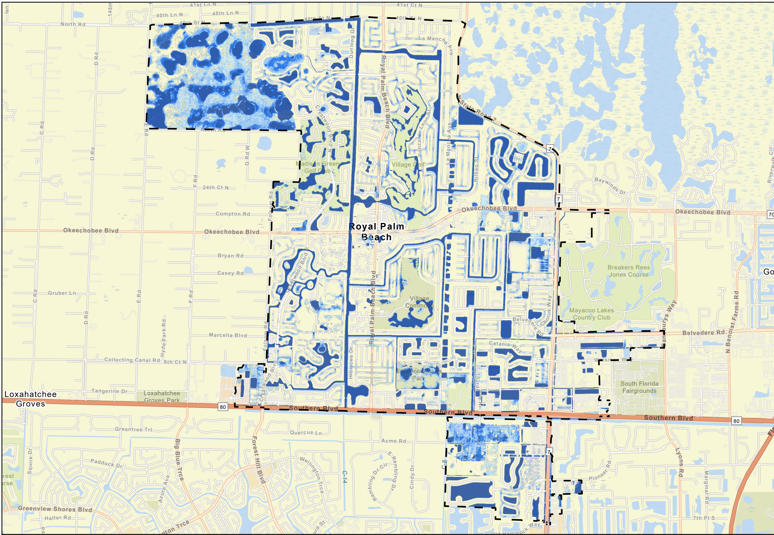
Proposed CIP Results Flooding Reduction 10-yr, 72-hr Design Storm for Alternative 1
