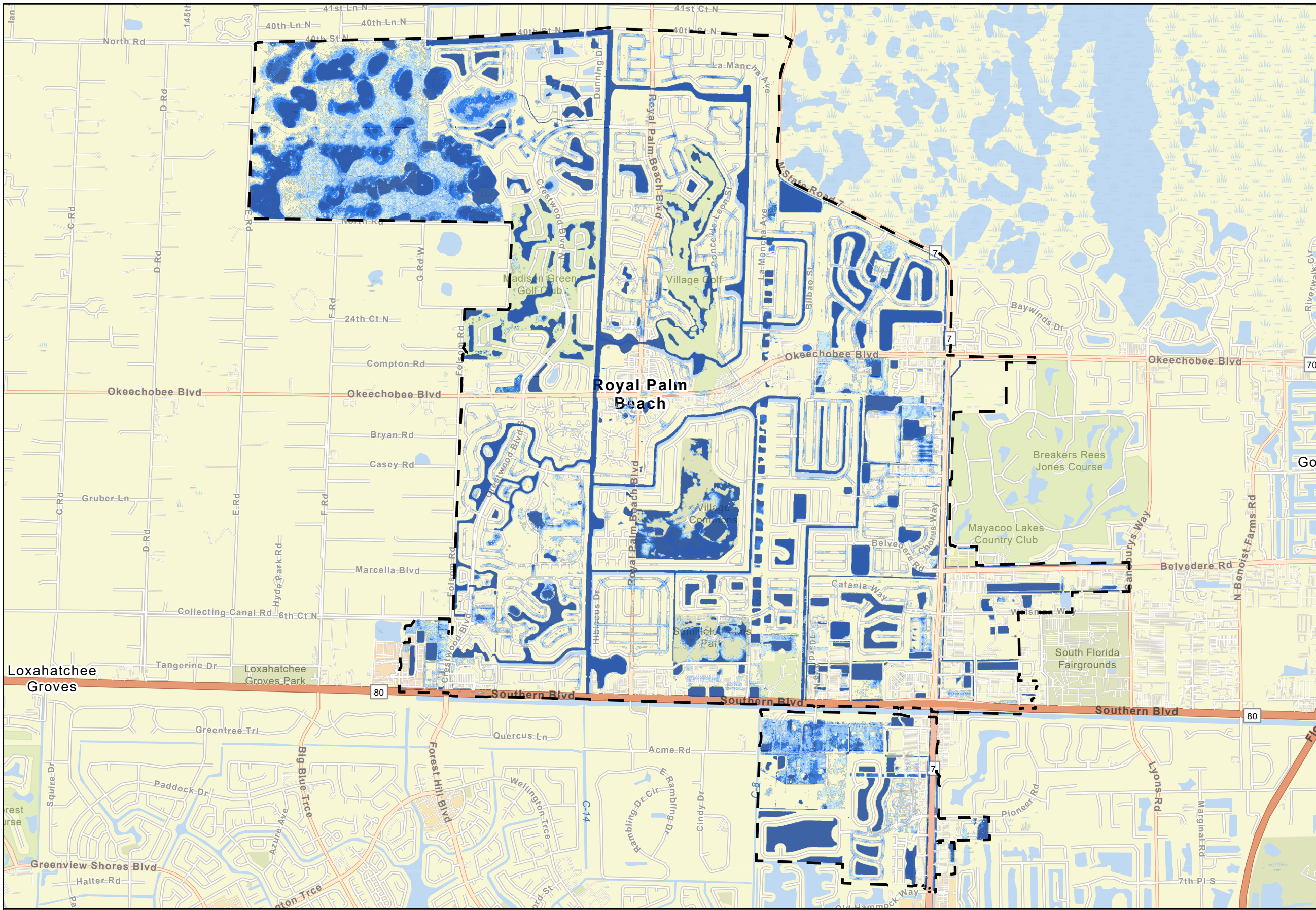
Proposed CIP Results Flooding Reduction 10-yr, 72-hr Design Storm for Alternative 1&4 Combined
