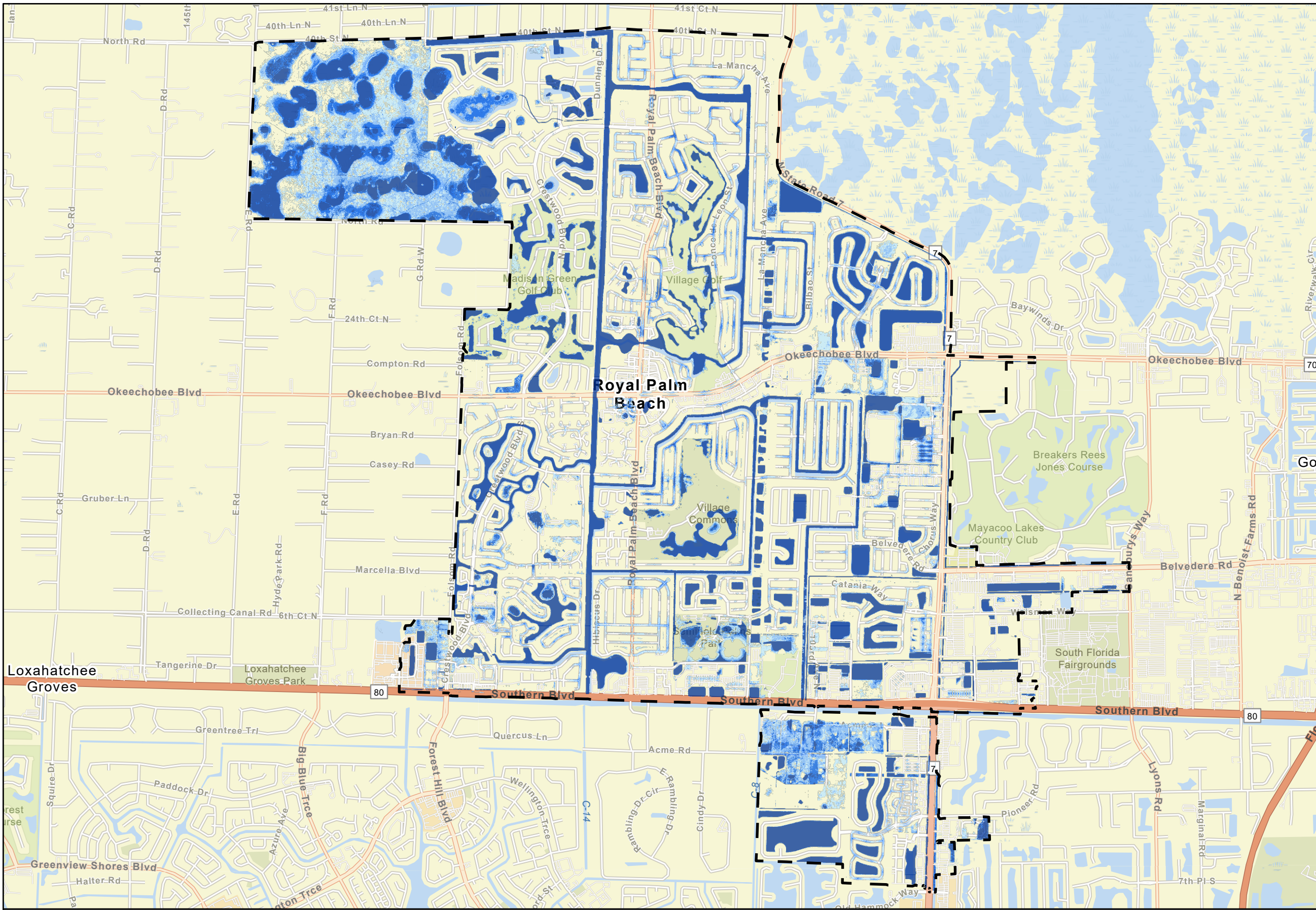
Proposed CIP Results Flooding Reduction 10-yr, 72-hr Design Storm for Alternative 2
