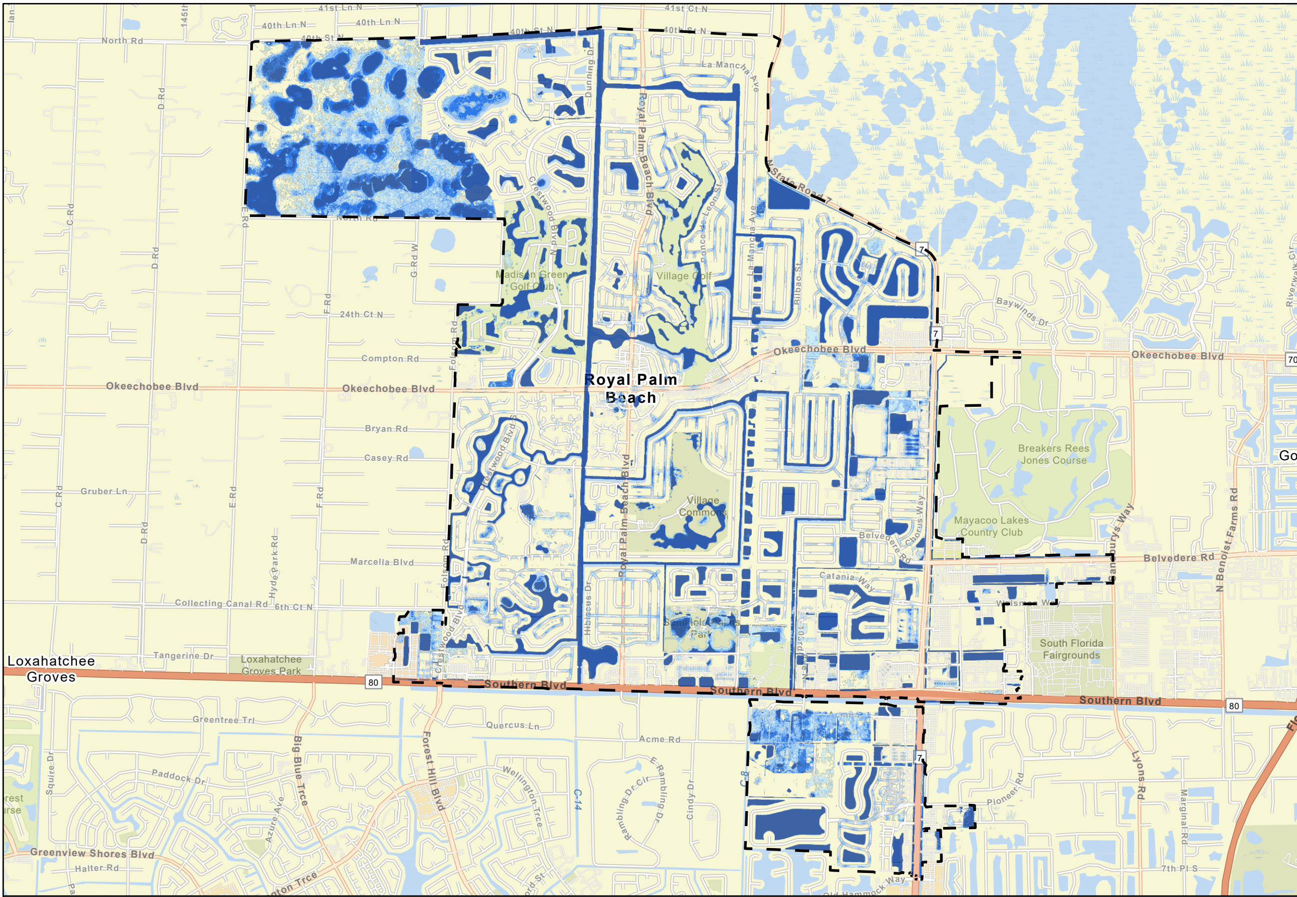
Proposed CIP Results Flooding Reduction 10-yr, 72-hr Design Storm for Alternative 1&2 Combined
