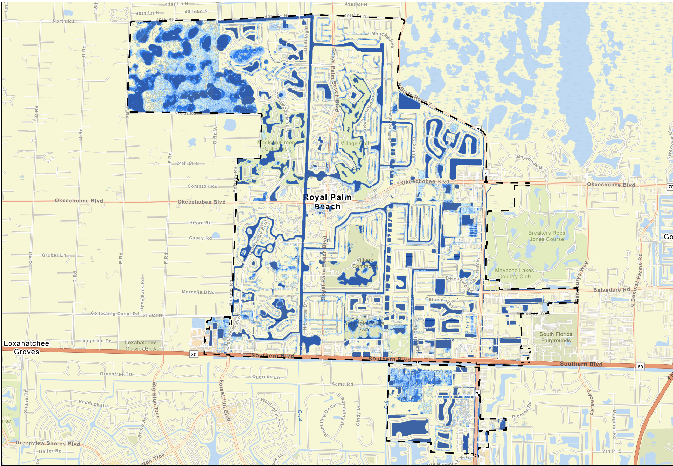
Proposed CIP Results Flooding Reduction 10-yr, 72-hr Design Storm for Alternative 3
