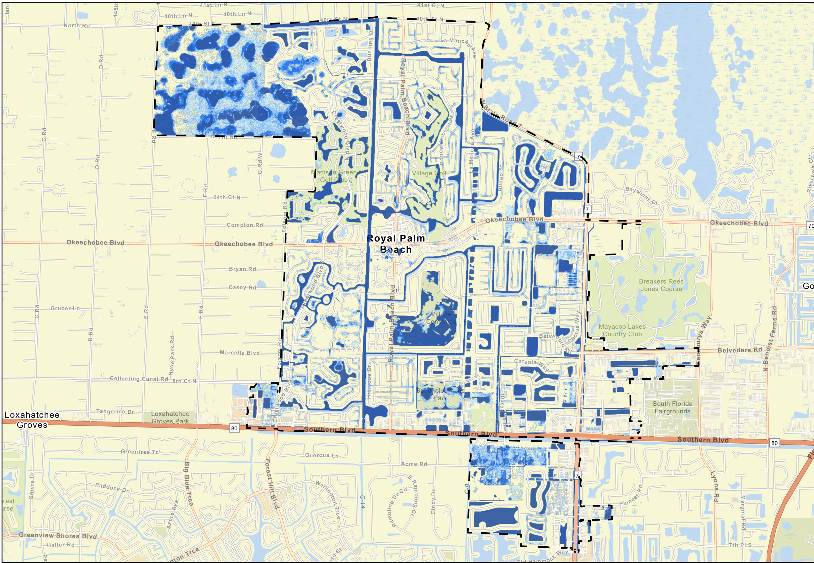
Proposed CIP Results Flooding Reduction 10-yr, 72-hr Design Storm for Alternative 4
