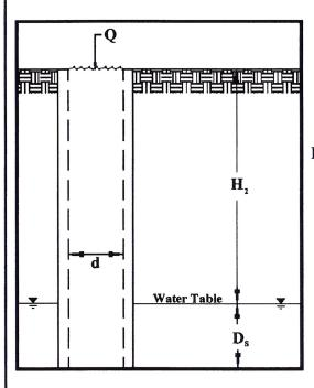
$$K = \frac{4Q}{\pi d(2H_2^2 + 4H_2D_s + H_2d)}$$
